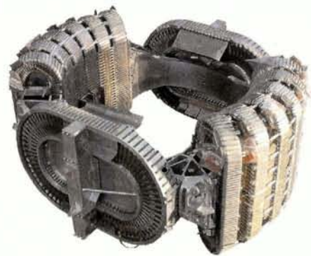
AMS - a 1.1 m clear bore actively-shielded dipole magnet for use in space
