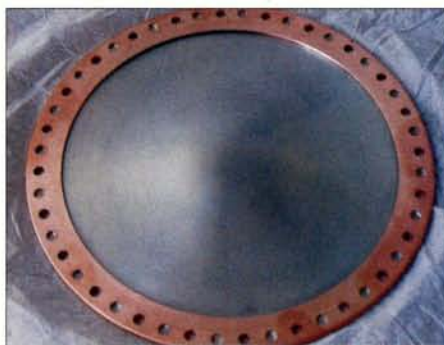
Custom-made beryllium RF cavity window, which leads to an improvement in the electromagnetic field by a factor of two.
