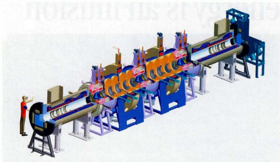
Engineering drawing of the MICE experiment, which is 15 m long and 3 m high. The beam enters through the time-of-flight counters at the left, goes through the spectrometers for momentum and angle measurements, then enters the cooling channel made of a succession of liquid-hydrogen absorbers and RF cavities embedded in a magnetic field.
