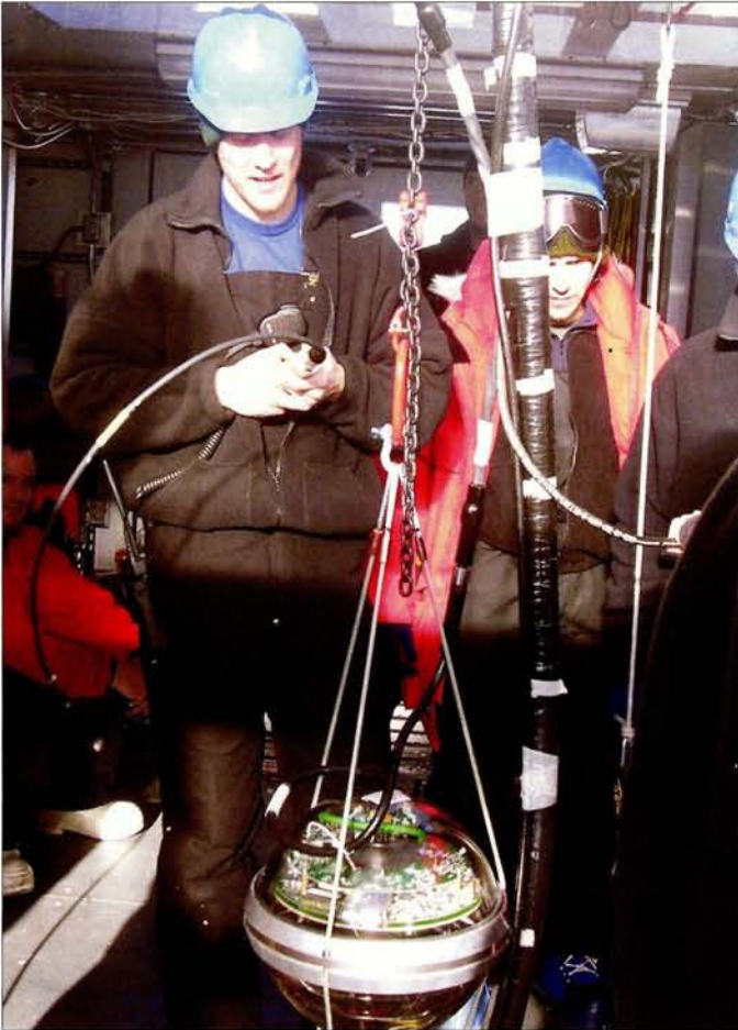
Fig. 2. The first digital optical modules are lowered into the hole.
